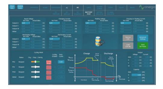
Battery Pack Testing This functionality enables the user to precisely control the charge, discharge and cycling of a Battery. Basic parameters include the charge/discharge current, fast charge and floating voltages while Advanced parameters add Energy (Ah) and Time as transition conditions. Profiles for each Battery technology can be saved and imported in .CSV files.
