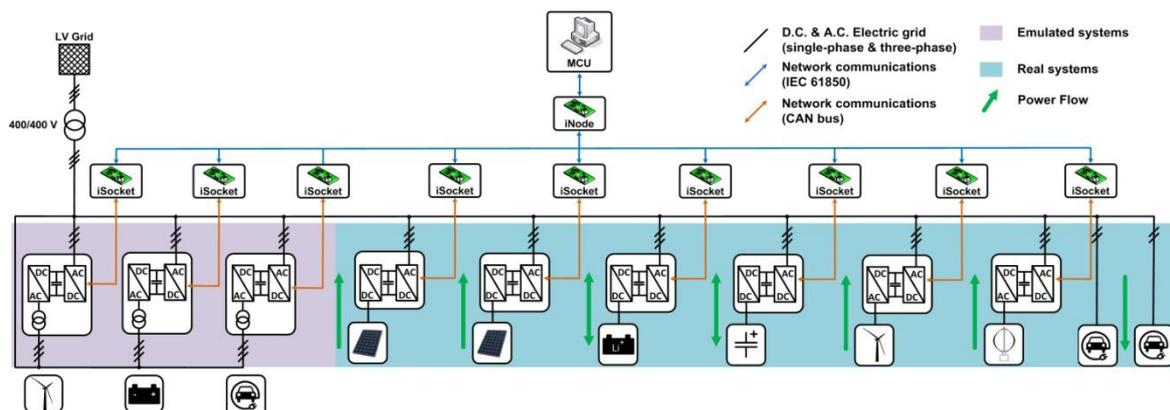
Fig. 1 IREC’s microgrid functional schematic.
