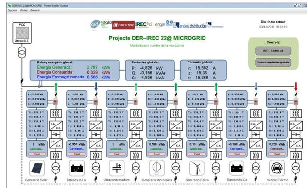
Fig. 6 IREC's SCADA.
