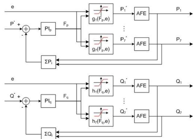
Fig. 5 Active and Reactive power closed-loop control.
