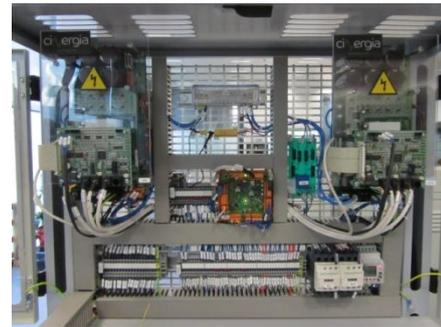
Fig. 3 Converters used in back-to-back configuration.
